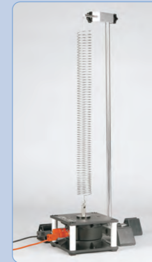
Experiment P 14 10 Longitudinal Standing Wave in Helical Spring
