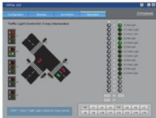
Traffic Light Control For 3-Way Inter Section
