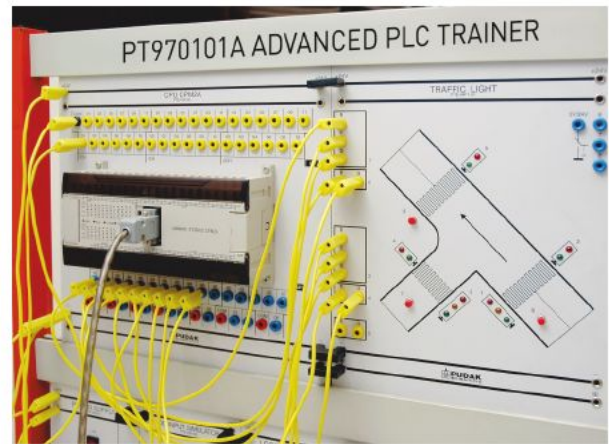
CPU CPM2A Omron [ PTE-033-02 ] with Model (Simulation) Plant
