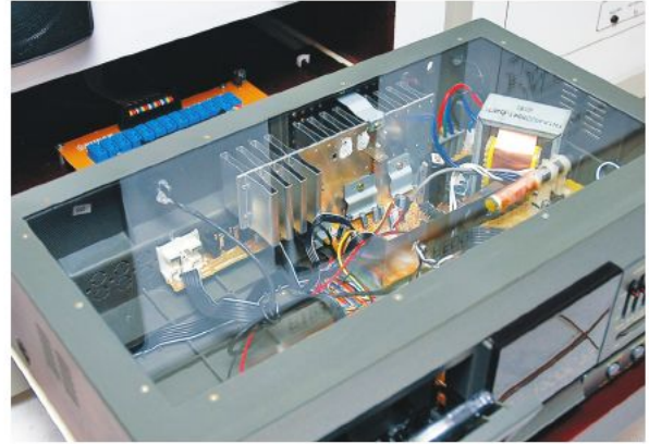
Transparent cover to make the circuit board viewable from outside
