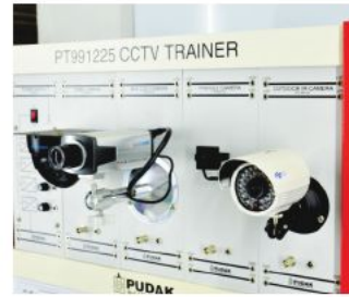
CCTV Cameras in Modular Panel System
